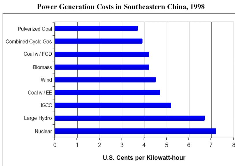
*Note: Coal w/ FGD is pulverized coal power generation with flue gas desulphurization (dry scrubbers); Coal w/ EE is pulverized coal power generation with environmental externality; IGCC is integrated gasification combined cycle<sup>15</sup>.*
